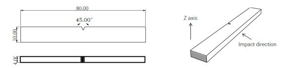
Fig 3. Impact testing specimen
