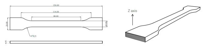
Fig 1. Tensile testing specimen
